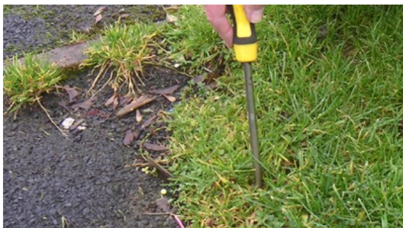
Probe detects hidden underlying hard surface
