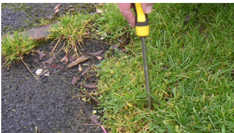
Probe detects hidden underlying hard surface
